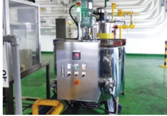
Oil Mixing Tank
