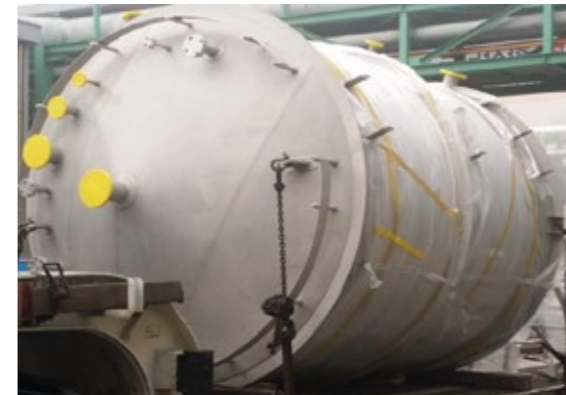
50m 3 Storage Tank
