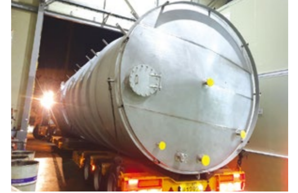
150m 3 Storage Tank
